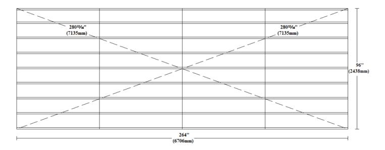
NB:- Floor joists run from gable to gable.
